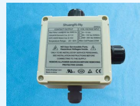
SR802 Dimension:100mm×100mm×65mm Voltage Max:180V~264V/AC 50/60Hz Resistive:25A (4KW) Inductive:2HP (1492W motor) Power:≤ 4000W Enclosure construction:ABS-impact resistant,UL94 V-0 Operation temperature:-10~50°C Water proof grade:IP43
